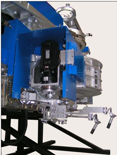
Shears can be turned to  $(0 \div 90)^{\circ}$  to the left and  $(0 \div 60)^{\circ}$  to the right (viewed against the molten glass flow)
